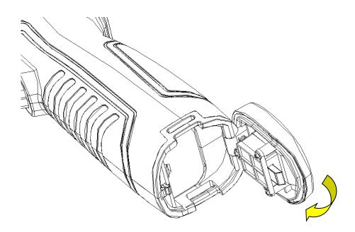
**! CAUTION:** Use only original manufacturer replacement battery. Use of incorrect battery may result in physical or electrical damage to the instrument due to incorrect voltage or physical size difference.
