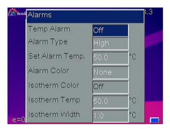
Press **Menu** key to activate the main menu. Select **Setup->Analysis setup** and press **Confirm** key to pop up the Analysis dialog box. User can set
