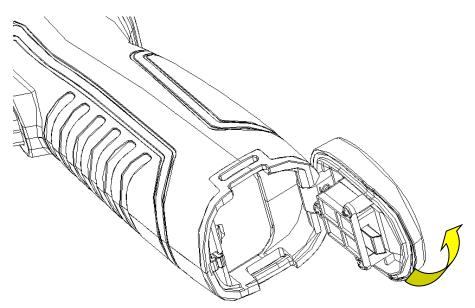
Insert the battery (the battery contacts must face into the battery compartment).
