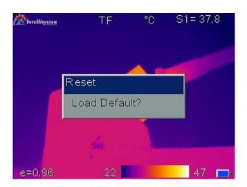
It is used for resetting factory defaults. Press **Menu** key to activate the main menu. Select **Setup->Default** and press **Confirm** key to open the **Reset** dialog box. Press **Confirm** key to reset the factory default. Press **C** key to cancel the reset operation. Appendix B indicates the detailed factory default parameter table.
